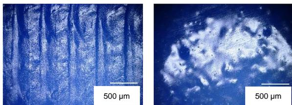
**Fig. 4** Left: Printed PLA component from the FDM process without a post process; Right: PLA part after the laser based polishing.
