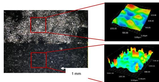
**Fig. 1** Comparison of the roughness from the surface of a printed SLM part (bottom) and the surface after the polishing process (top).
