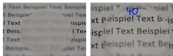
**Fig. 2** Left: Fused silica slice before the polishing process; Right: Fused silica slice after laser polishing.
