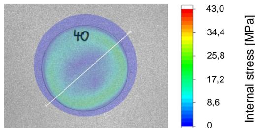
**Fig. 3** Internal stress of a laser polished fused silica slice.
