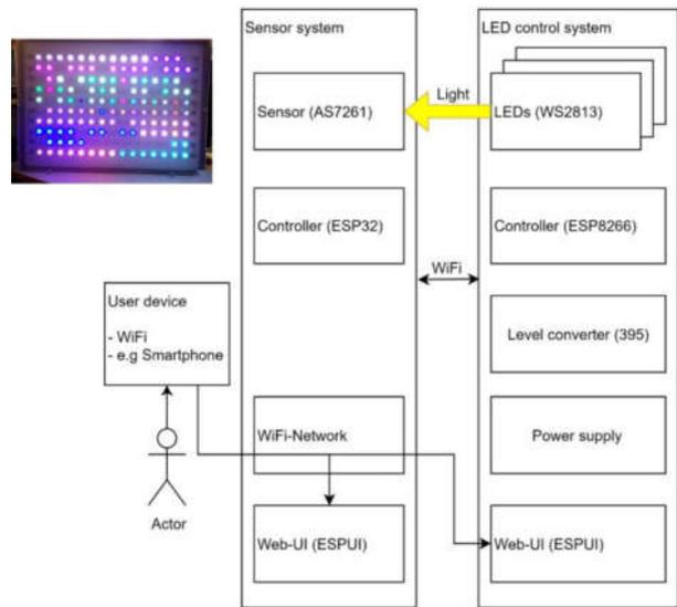
**Fig. 6** Block diagram of large area matrix RGB LED lighting with connectivity for remote control and animations (e.g. moving white clouds over blue sky) as well as illuminance and color supervision.
