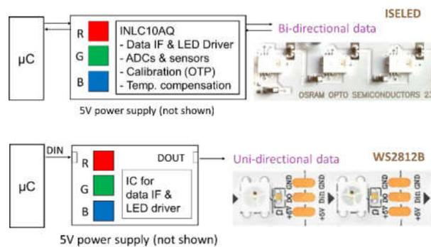
Fig. 2 The two evaluated concepts [2] of RGB LEDs with integrated drivers and data interface: automotive optimized ISELED (top, [1]) and WS2812 (bottom) as example for consumer electronics and limited commercial use.
