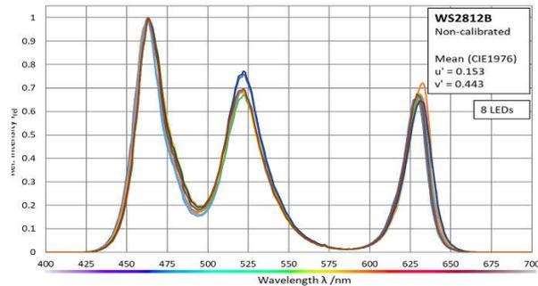
**Fig. 4** Example spectra of WS 28123B measured and visualized for 8 neighboring LEDs. ISELED spectral characteristics see [3].
