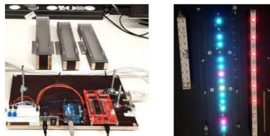
Fig. 3 Prototype system for evaluation of the two concepts: Microcontrollers and housings with different diffusers (left) and screenshot of a movie of fast dynamic animations (right) such as chaser/running light.
