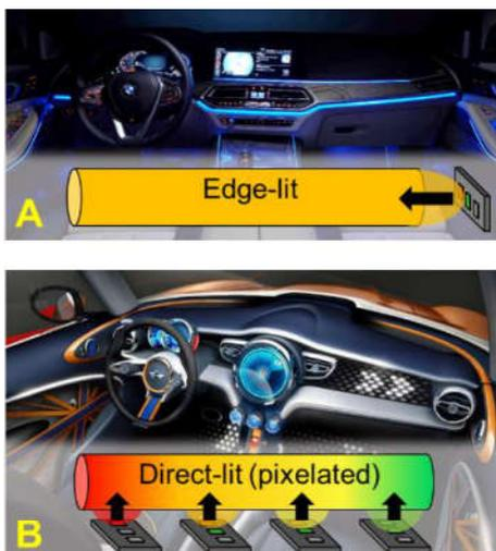
Fig. 1 Today’s automotive interior lighting by edge light (A) and future advanced pixelated lighting (B, direct-lit).
