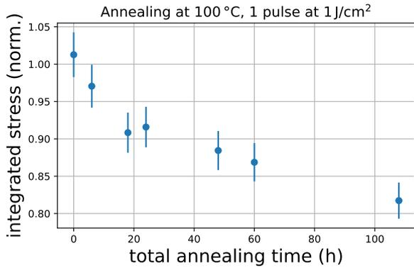
**Fig. 2** Annealing at 100°C in ambient air causes a faster decrease of the integrated stress with time than at room temperature. The obtained integrated stresses for irradiation with one pulse at 1 J/cm<sup>2</sup> after different total annealing times are normalized by the values for a sample kept at room temperature.
