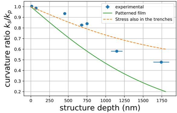
**Fig. 3** Irradiation with a line pattern leads to an anisotropic deformation of the sample. The curvature ratio  $k_s/k_p$  of curvatures in directions across and along the lines is plotted in dependence on the depth of the line pattern. The experimental results are compared to the Theory of Wikström et al. [3] for a stressed film patterned into lines and to Eq. (1), which additionally considers the generation of a stress in the trenches of the line pattern.
