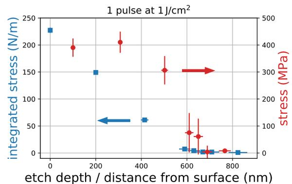
**Fig. 1** For irradiation with one pulse at a fluence of 0.99(5) J/cm<sup>2</sup>, we measured the integrated stress (left ordinate) in dependence on the thickness of removed material by etching in KOH solution. From this data, we calculated the stress distribution in direction normal to the surface (right ordinate).
