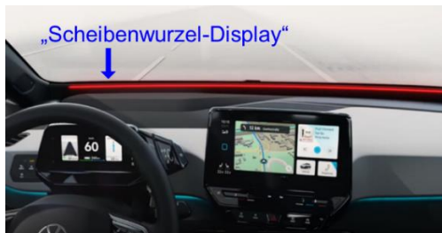
Fig. 1 Light guide showing red of VW ID.4 [1] with RGB LEDs between dashboard and windshield; Source: VW.
