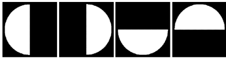
Fig. 2 Illumination patterns generated on the LED Array to capture differential phase images.
