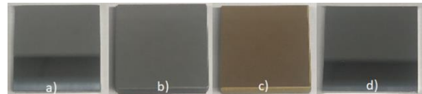
Fig. 2 Pictures of four characterised mirror coatings a) Al b) protected Ag c) protected Au d) Ir
