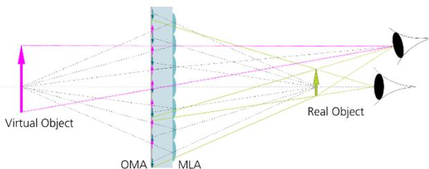
**Fig. 1** Working principle of the lightfield display. As the viewer moves their gaze, the objects seem to float about following the gaze or in the opposite direction.
