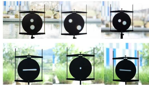
Fig. 5 Lightfield device displaying the double-sphere (top) and piercing stick (bottom) motif under various viewing angles.
