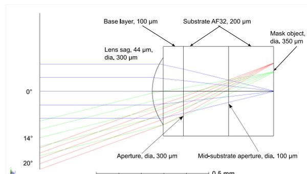
**Fig. 3** Layout of single channel of the regular MLA with ray traced backwards from  $20^\circ$  field towards mask plane.
