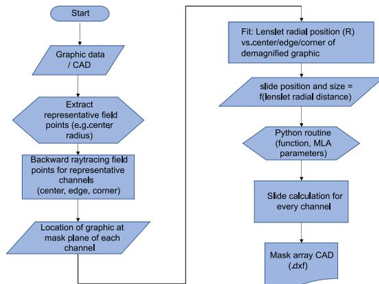
Fig. 4 Flow-diagram for analytical mask generation.
