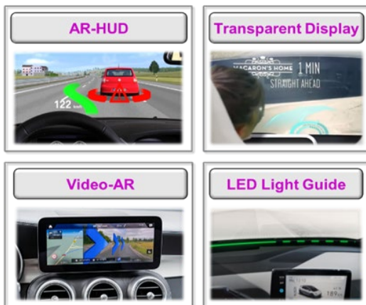
Fig. 1 Approaches to present augmented information to drivers and passengers by different types of displays; Sources: BMW, Saint-Gobin, Mercedes, Volkswagen.
