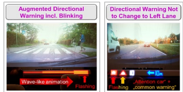
Fig. 7 Examples of dangerous situations: Pedestrian enters road (left) and navigation directs to the left lane (right), which is occupied by a car. Subjects rated these examples as being very helpful to raise traffic safety.
